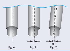
Typically when manufacturing a roller bearing, the alignment of the grinding tool to the component is critical.
