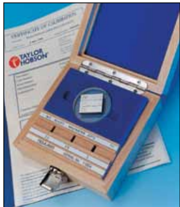
Figure 62: Gauge Block Calibration Standard
