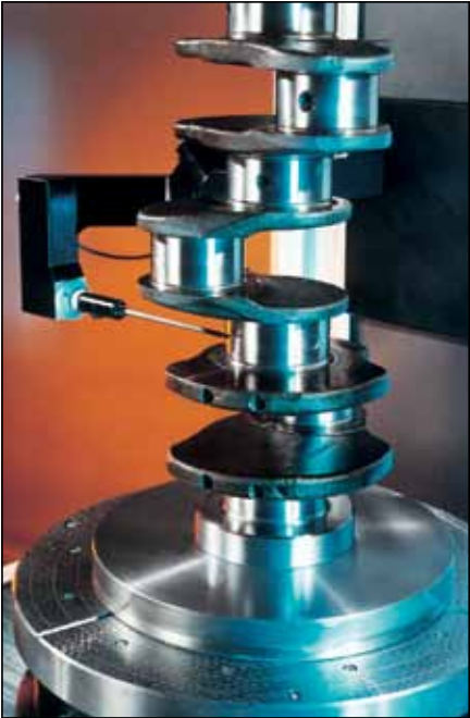
Figure 71: Talyrond instrument mapping a crankshaft oil hole
