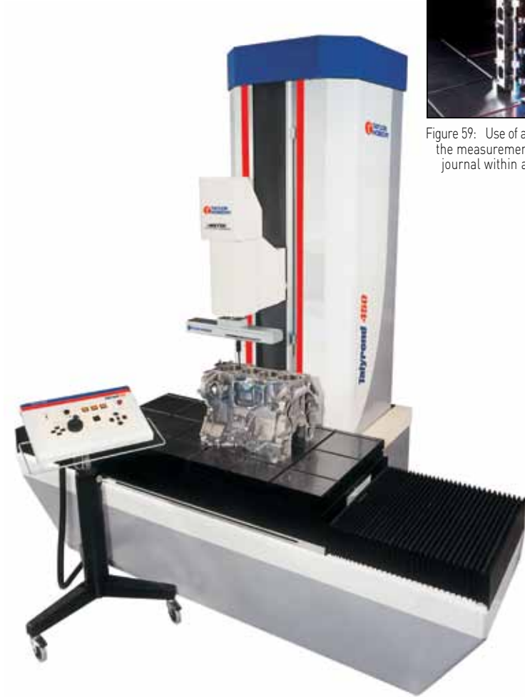
Figure 58: Talyrond 450 is an example of a rotating pick-up type roundness instrument
