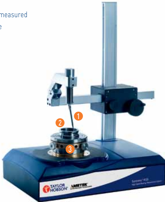
Figure 17: Typical roundness instrument uses a precision spindle to assess departures from a true radius
