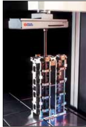
Figure 59: Use of a drop-arm enables the measurement of a camshaft journal within a cylinder head
