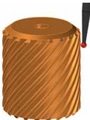
Figure 69a: Example of interrupted surface
