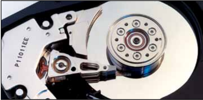
Figure 76: Hard Disk Drive Bearing assembly
