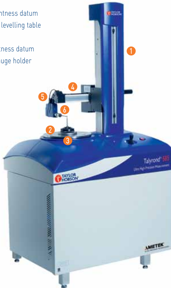
Figure 37: Fully automated precision roundness and form measuring instrument
