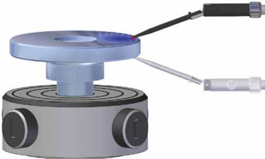
Figure 82: Measuring Wall Thickness Variation on a brake disc
