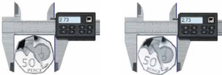
Figure 5: Although the radius varies, diameter of a British 50 pence coin remains constant
